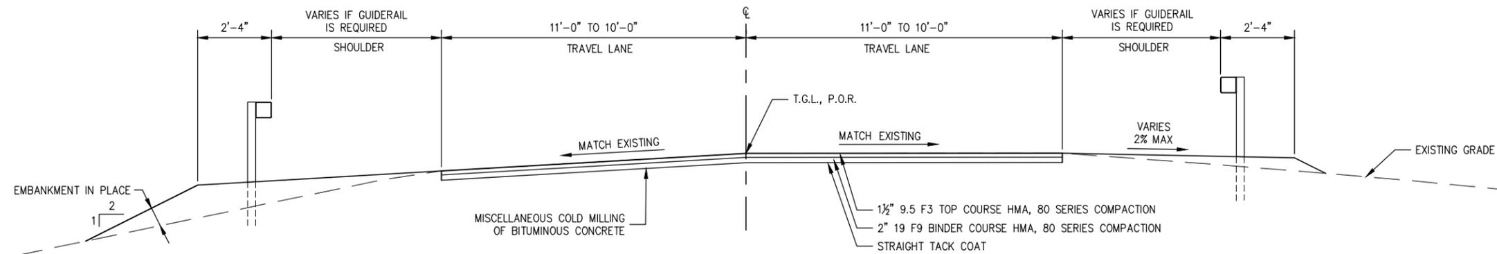
TYPICAL MILL AND OVERLAY SECTION
